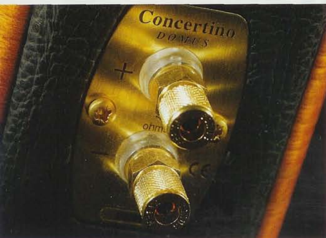
Both drivers are fed via a single pair of gold-plated binding posts with 4mm sockets
